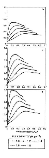
Fig. 3. Thermal diffusivity of soil in the function of soil moisture. Austria: a) profile Wiselburg, b) profile Fuchsenbigl; Czech Republic: c) profile T11P, d) profile T12P, e) profile T13P; Poland: f) profile Forest, g) profile State farm.
